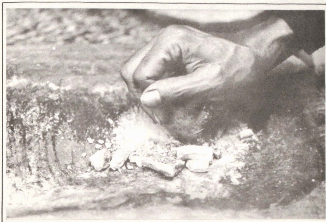
Crushing and grinding the resin ( sāl dhūp ) with the help of a round stone ( lvahā )
