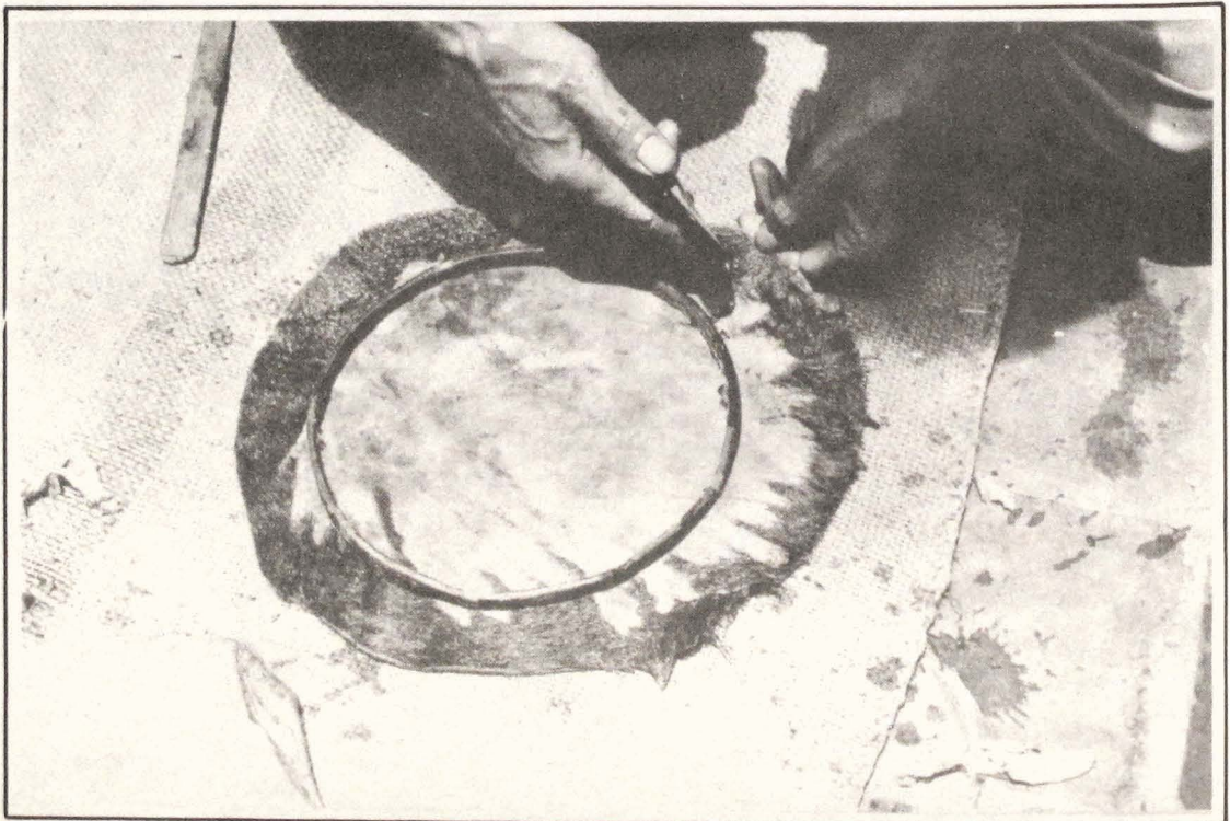
Cutting the wetted Nāsaḥ -hide into shape ( cāḥ lakegu or cāḥ utigēkegu )
